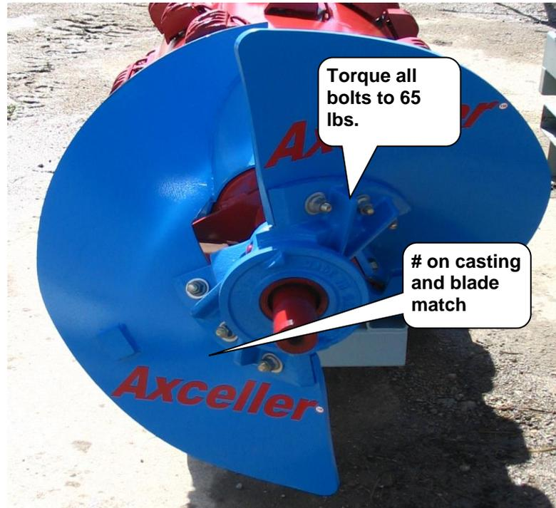
Flighting should have 1/8" to 1/4" clearance from kidney. Adjust using existing spacers supplied with combine between rotor & Kidney bearing
